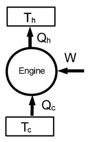
A heat pump can be used for heating. The engine requires the input of work [e.g., by plugging it in an electric outlet] and removes heat  $Q_c$  from cold reservoir [outside] and delivers heat  $Q_h$  into hot reservoir [inside the house]:  $Q_c + W = Q_h$ . Coefficient of performance is defined as the ratio of the gain
